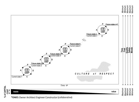
Figure 1: The continuous improvement process of lean construction (after Rybkowski et al. 2013, Figures 4 & 5, p. 88).
