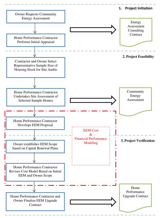
Figure 2: Typical Energy Improvement Retrofit Process
