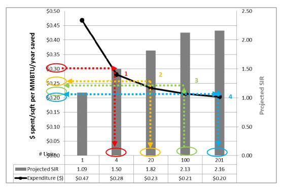
Figure 6: Projected range of savings-investment ratios and cost intensity per achieved energy savings for air sealing and insulation measures
