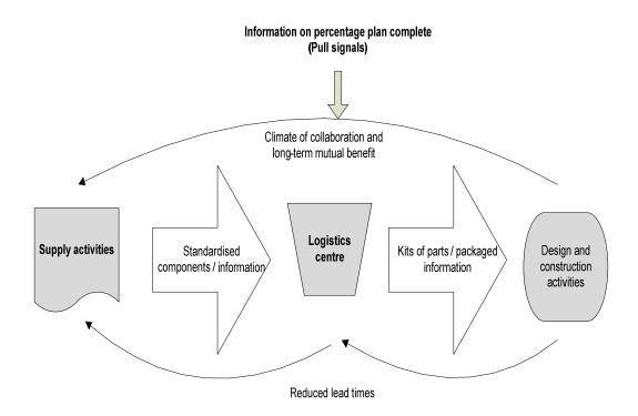
Figure 1: Lean supply system suitable for construction logistics management (source: Terry and Smith 2011: 147).
