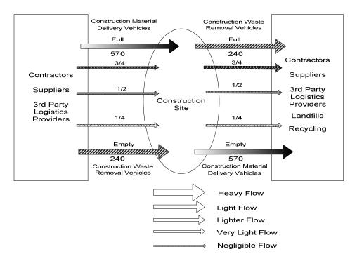
Figure 3: Integrated materials delivery and waste removal logistics
