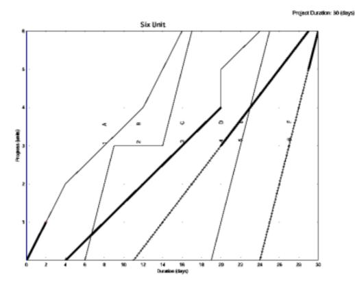
Figure 3. RSM Graphical Schedule for the Six-unit Project
