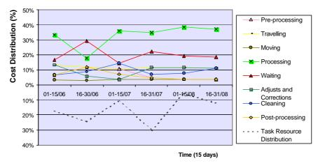
Figure 6: Temporal evolution of cost distribution - concrete supplying.
