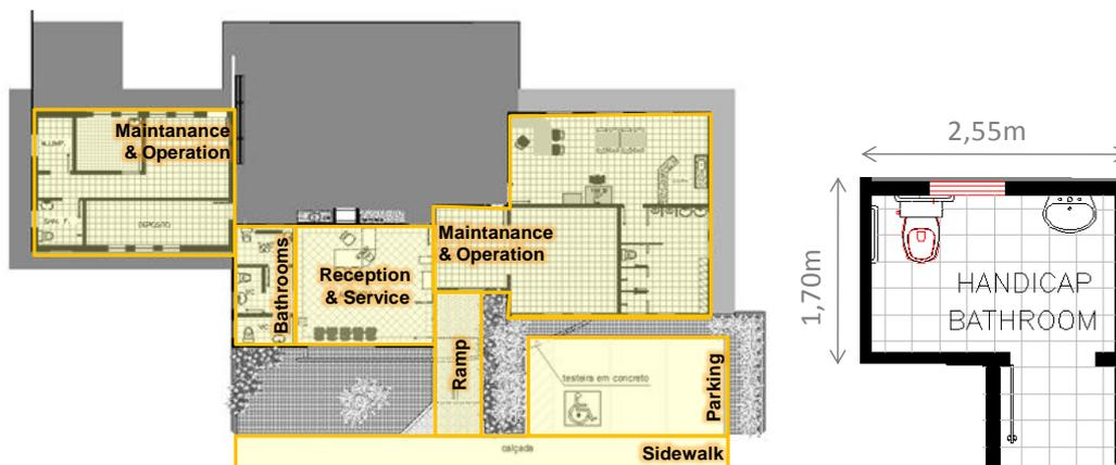
Figure 3 (A): Building design and activities in each area. (B): Handicap bathroom design and dimensions. (ENERGY PROVIDER COMPANY, 2005).
