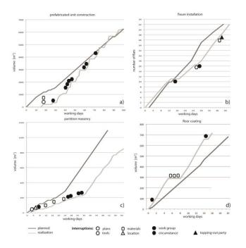
Figure 2: The planned and actual work rate in four cases of the set B. Disruptions and making-do effect is seen in the work rate. When pre-requisites are in order, the planned work rate is achieved. When pre-requisites are not in order, neither is the work rate as planned.
