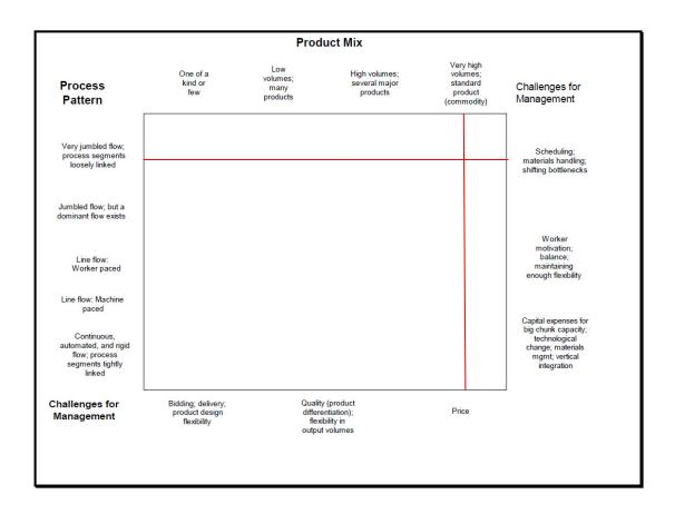
Figure 2: Manufacturing Characteristics (adapted from (Ballard and Howell 1998)
