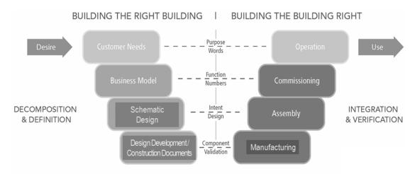
Figure 1: System "V" diagram for the building industry (Rubel, 2012)
