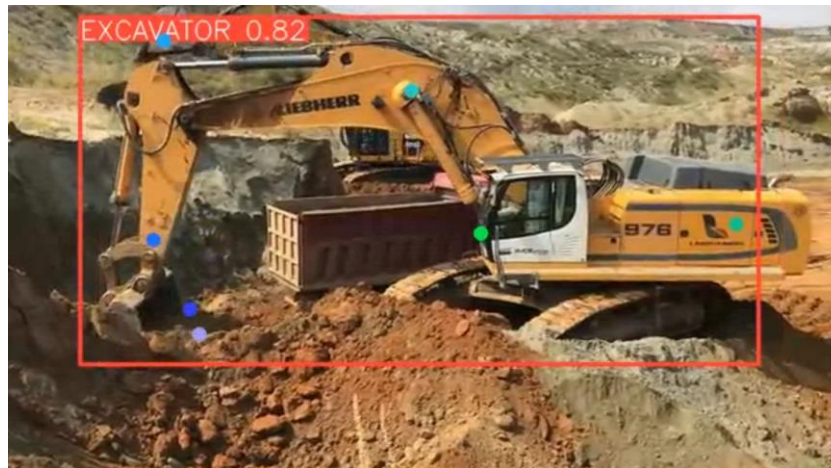
Figure 3 Example of a Computer Vision Model Detecting Excavators and Key Points
