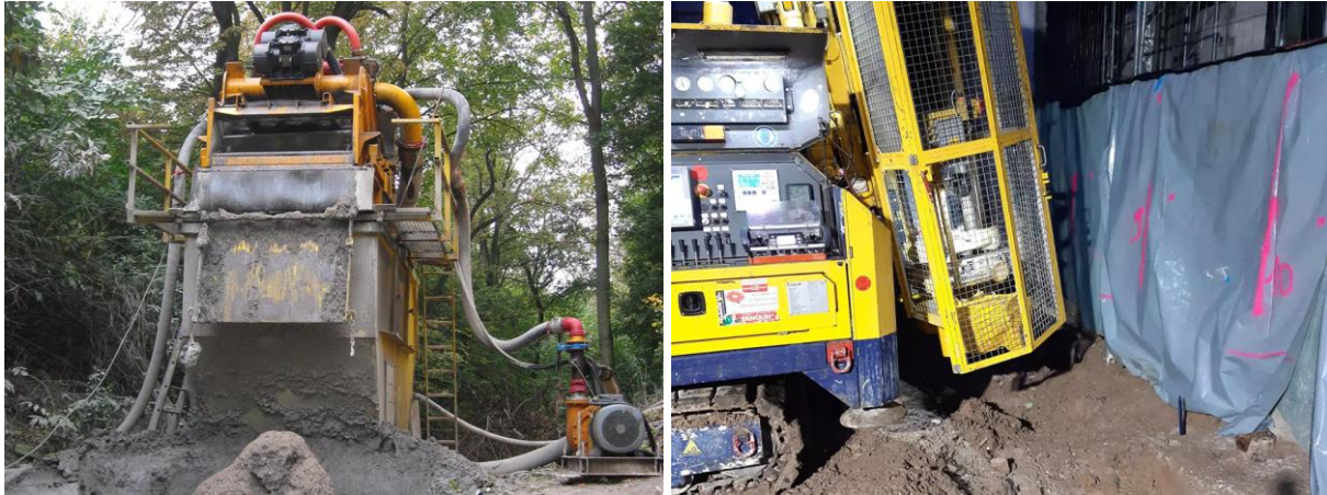
Figure 2: Schematic representation of the separation plant for processing the backflow suspension (Keller, n.d.a, n.d.b)
