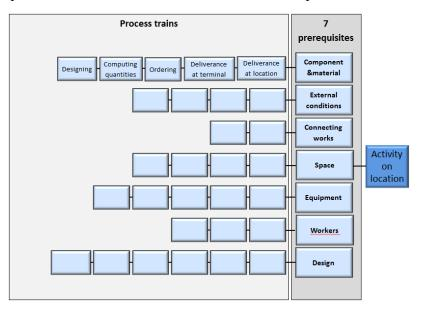
Figure 2: "Process trains" (each activity has process sequences, sets of actions, which must be completed in order for each of the seven prerequisites to be sound)
