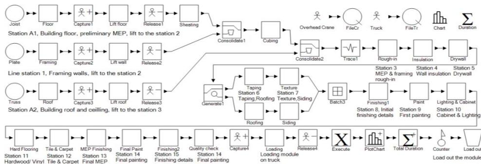
Figure 7: Future-state VSM simulation model
