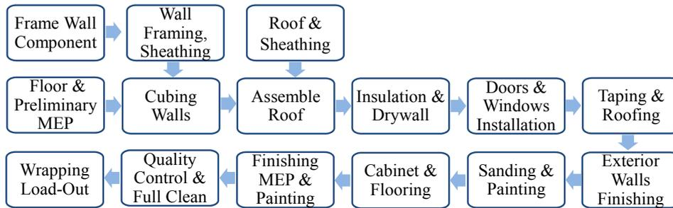
Figure 1: Production tasks layout of a modular building
