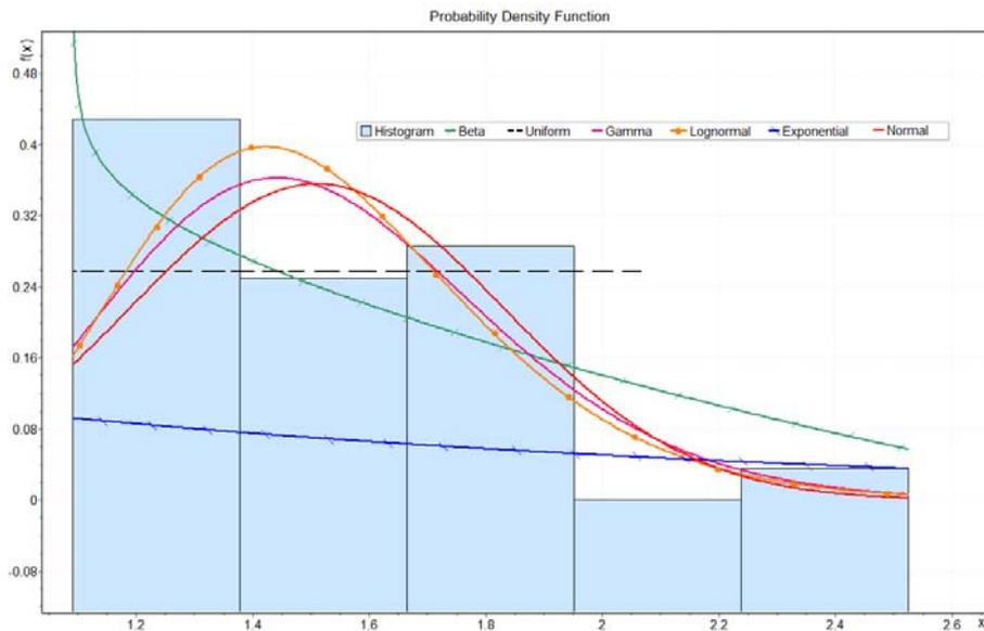
Figure 4: Probability Density Function of exterior wall productivity rate
