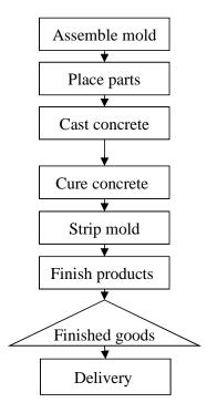
Figure 1: Precast production process
