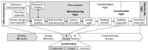
Figure 3: Time frame for the typical building project with a simplified model of activities during design, manufacturing and commissioning.
