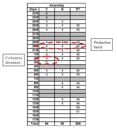
Figure 3.Structure assembly batches – stage 1 (C=columns; B = beams; RT = roof tiles)
