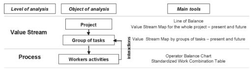
Figure 1.Preliminary proposal – sequence of analysis for continuous flow implementation in construction (Bulhões et al, 2005)
