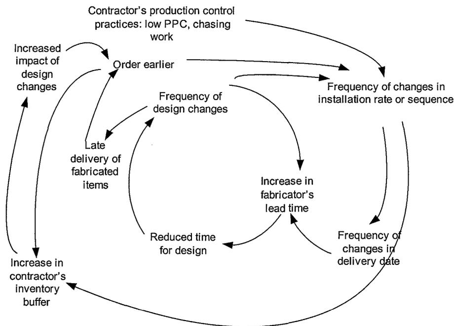
Figure 2: Interdependence of demand variability and fabrication lead
