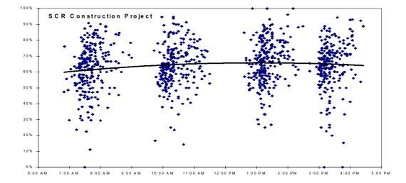
Figure 2: Variability of productive workforce utilization. Data points are average productive utilization of overall workforce of approx. 350. The shift had 3 organized break periods (during which no data were gathered).
