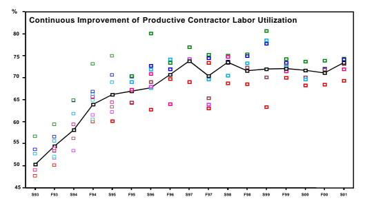
Figure 3: Continuous work process improvement at major utility from 1993through early 2001. Data points represent average productive labor utilization achieved at major plant modification and outage construction projects. Trend line shows system-wide average; the sudden drop in 1997 corresponds to a change of contractor.
